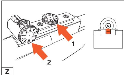
Your airgun is equipped with an adjustable rear sight for both elevation (1) (up-down) and windage (left-right) (2).
