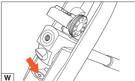
Blued parts as barrel and compression cylinder should be protected from rusting. Maintain protection by wiping these parts with a lightly oiled pad.
