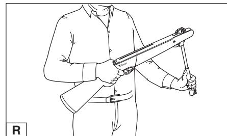
Grasp barrel behind the front sight and pull downward until it stops. You will hear an audible click of the trigger mechanism lock when the pressure is released. You must control, and not release, the barrel under strong resistance until the audible click is heard.
