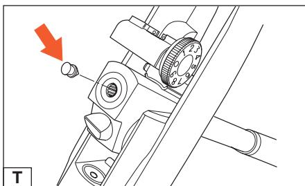
Move barrel back to its original locked position.
