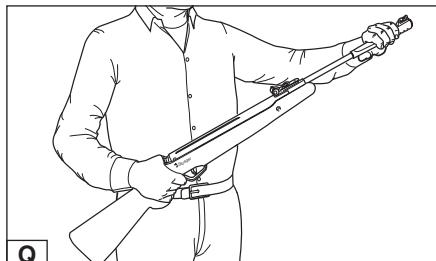
With one hand grasp stock at the pistol grip. Holding the rifle firmly, tap barrel behind front sight in order to break locked position (fig. R).
