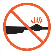
Always check the barrel prior to loading to ensure that it is clean and free from obstructions. **Firing against an obstruction can cause a dangerous build up of pressure and might injure yourself or others nearby.** If you hear an unusual noise when shooting, stop firing immediately, engage the manual safety and unload the airgun. Make sure the barrel is free from any obstruction.
