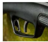
The trigger comes to a definite stop when it reaches the end of first-stage travel, but second-stage trigger-pull was a little hefty out of the box
