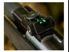
The rear fibre-optic sight is only supplied in green, but the sights can be adjusted for windage and elevation by turning the finger-friendly dials
