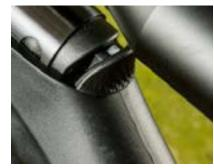
The shotgun-style safety catch is automatically set when the rifle is cocked, and is disengaged by thumbing it forwards
