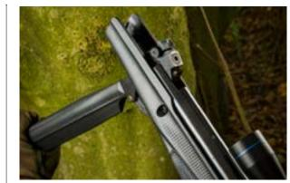
given the top of the shroud a sharp tap with the palm of your hand to release the barrel, the RX20 is surprisingly easy to cock
