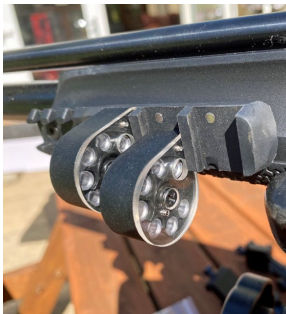
BELOW RIGHT: The magazine slots in easily and is held there via a magnet
